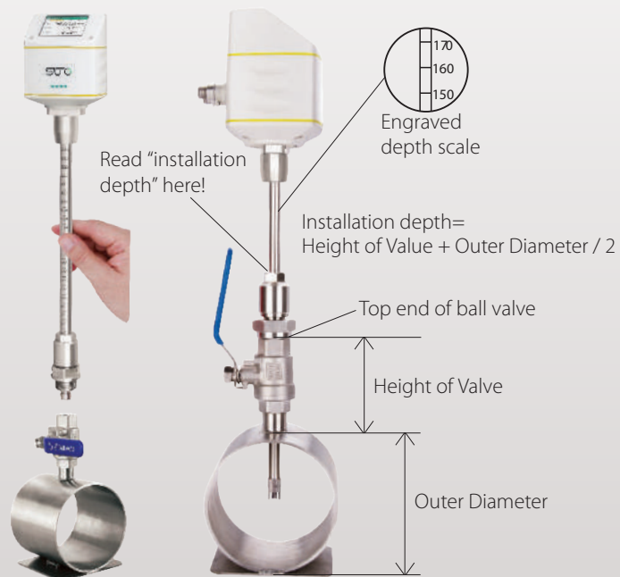
S430 Installation through a ball valve
